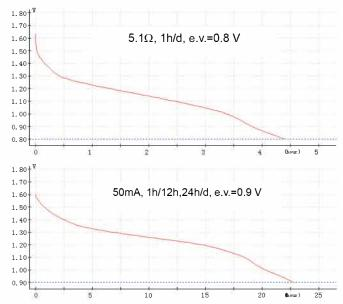
1) Store period before test shall be under 20±2°C, RH 55±20% within 30 days of manufacture.
